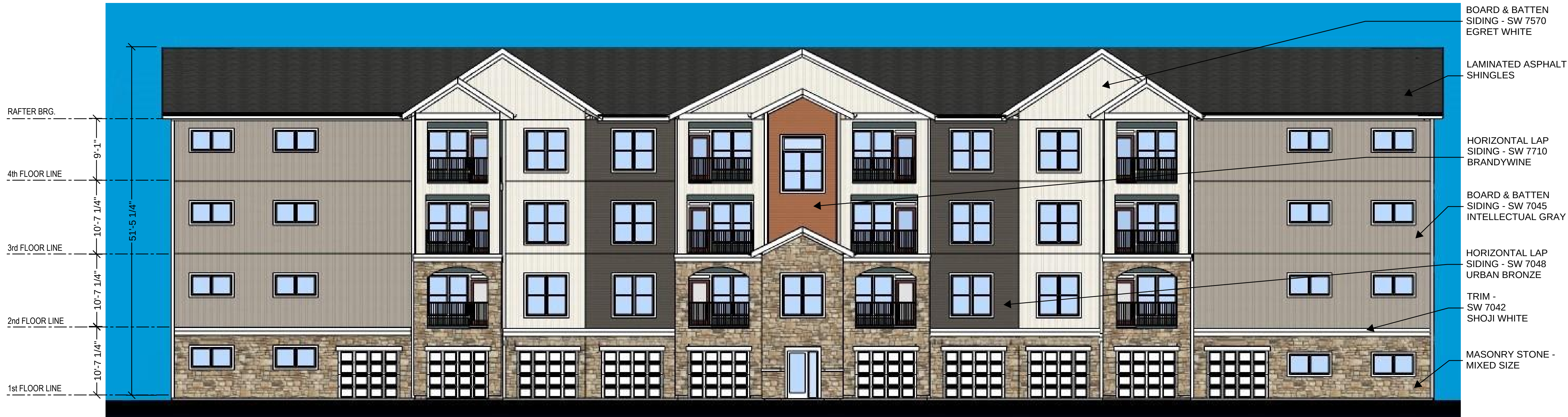
4-STORY APARTMENT BUILDING | FRONT ELEVATION
