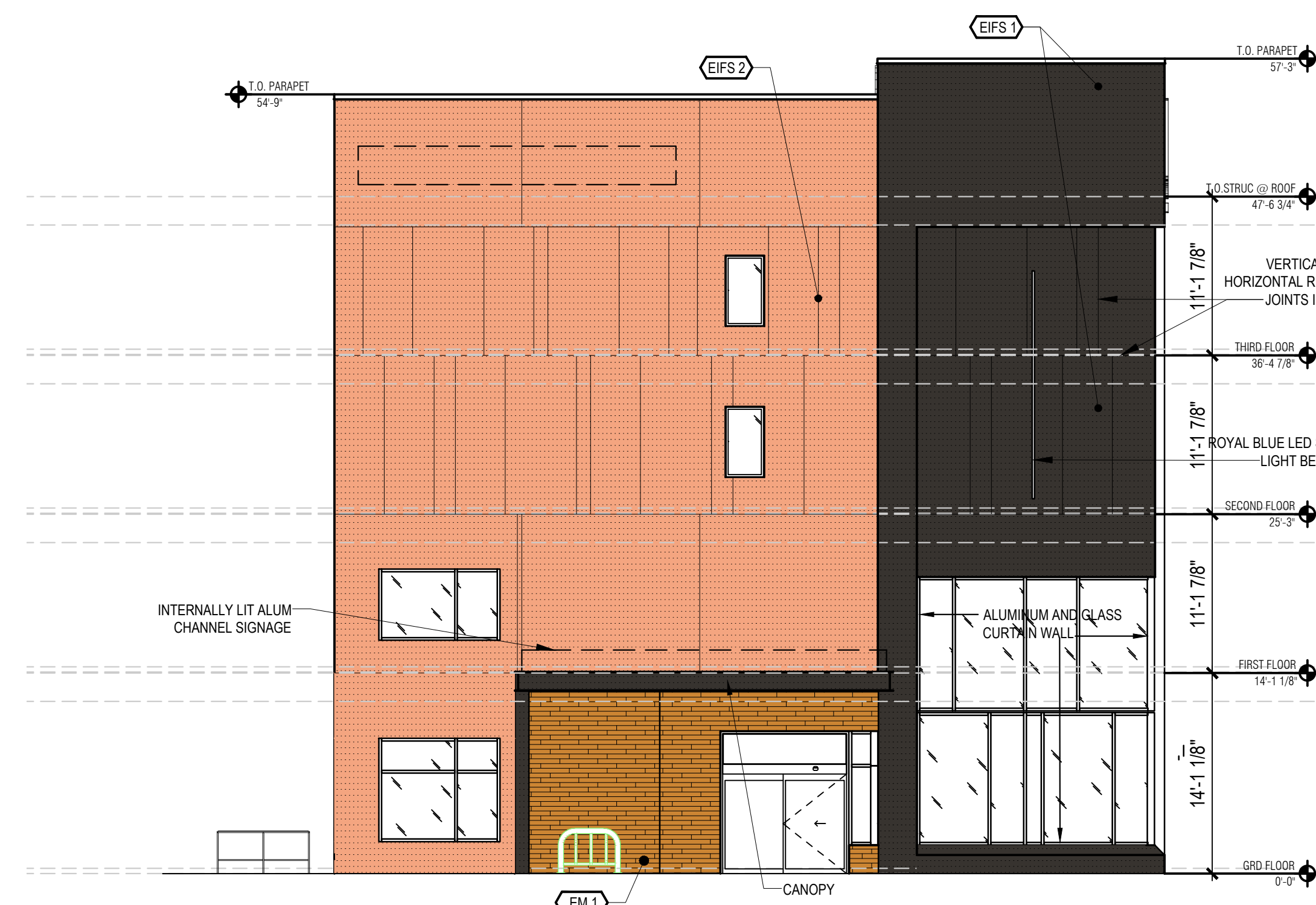
02 WEST ELEVATION - MAIN ENTRANCE A5.00 SCALE: 1/8" = 1'-0"
